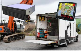
The Service vehicle receives Orders via Wireless communication (Wi-Fi / LTE). All Service orders are in que with priorities. When Service have taken place, the Computer sends report to Server. Print on paper is either on Vehicle installed printer or Office-printer thru Wi-Fi (when passing the office). All applications are supplied by third part.
