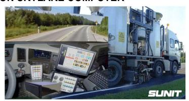
**SUNIT-FDC serial computers** base on our 1-DIN sized geometrical designed cast aluminium technology and purpose-designed conformal coated solid-electronics.
